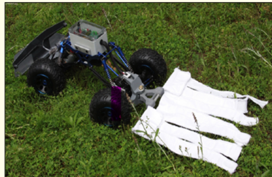
Figure 4: Image of tick bot, consisting of the robotic car and a drag cloth [10].
