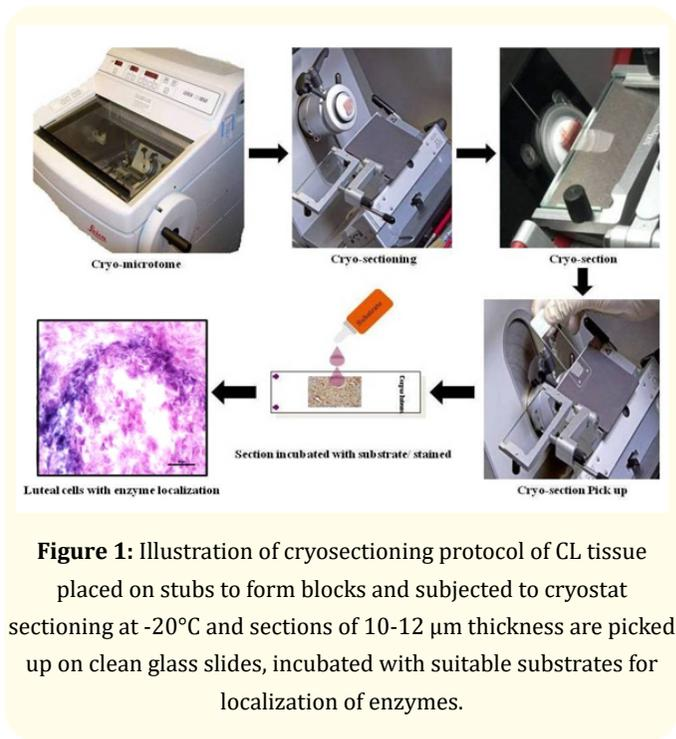
**Figure 1:** Illustration of cryosectioning protocol of CL tissue placed on stubs to form blocks and subjected to cryostat sectioning at -20°C and sections of 10-12 µm thickness are picked up on clean glass slides, incubated with suitable substrates for localization of enzymes.
