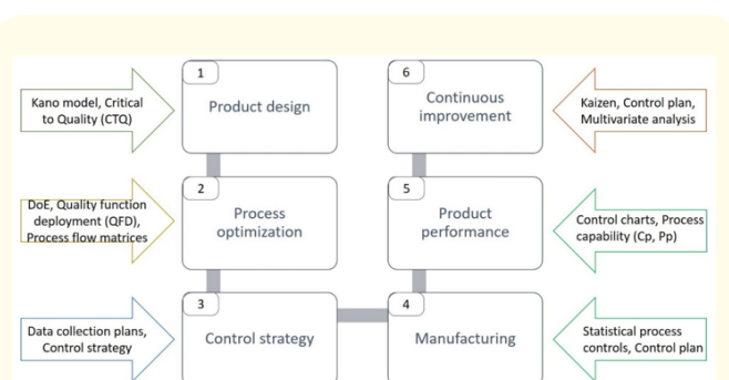
Figure 1: QbD framework with tools and techniques to be used at various stages for pharmaceutical drug product development.
