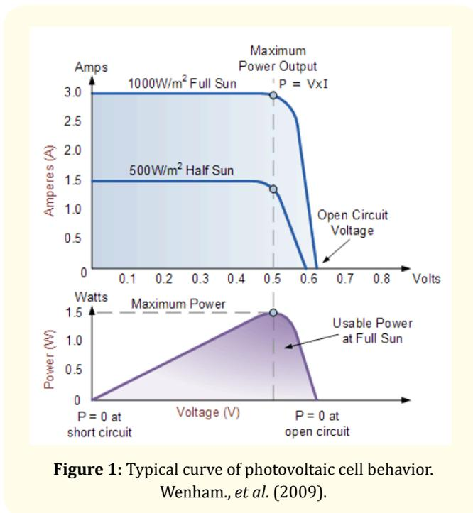
**Figure 1:** Typical curve of photovoltaic cell behavior. Wenham., *et al.* (2009).
