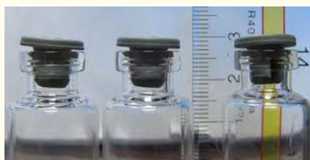
Figure 10: Improper Rubber stopper fitment cause Lyo product Failure.
