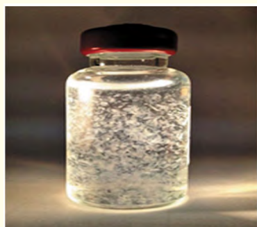
Figure 1: Example of Delamination in Glass Vial.
