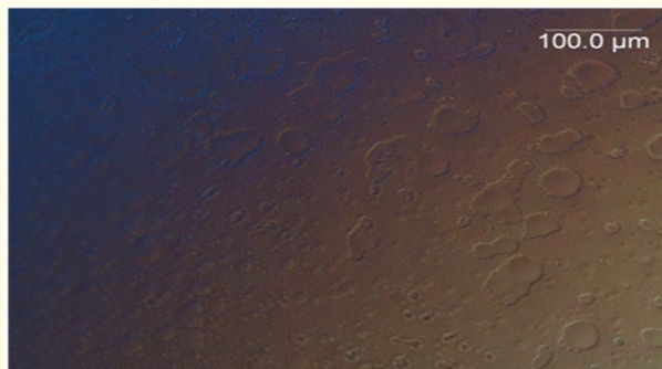
Figure 4: Glass delamination under the Carlton Microscope.
