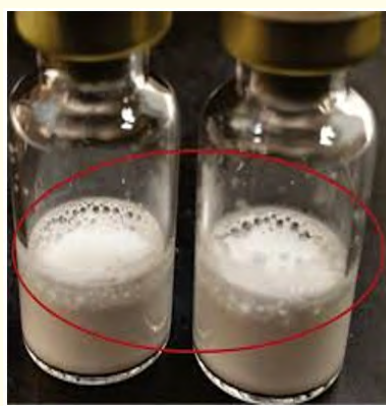
Figure 9: Excess moisture into the vial and improper Lyo cake.
