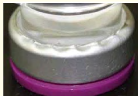
Figure 11: Improper crimping of flip-off seal cause failure of seal integrity test.
