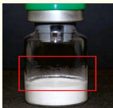
Figure 8: Seal Integrity Problem and Failure of Lyophilized Product.
