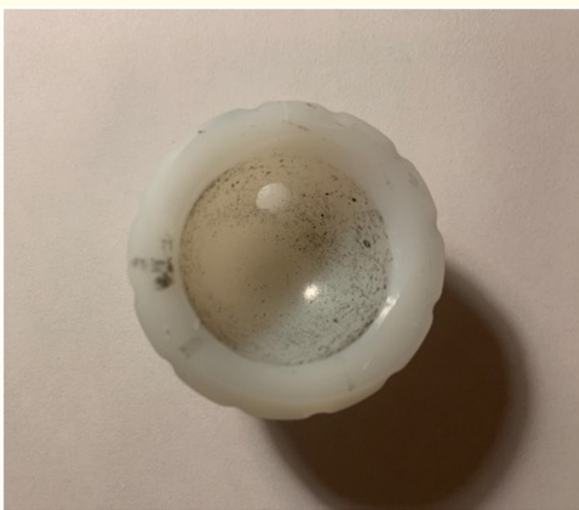
Figure 4: Black particulates of ceramic embedded in the original polyethylene liner acting like sandpaper on the femoral head.
