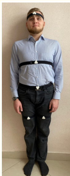
Figure 1: Starting position for the examination. 5 Notch motion sensors are installed on the examined person
