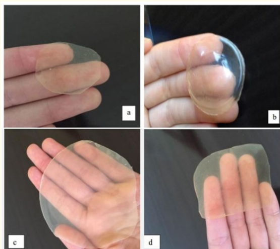
Figure 5: Membranes prepared using the brushstroke and deposition techniques, in (a) M1 - brushstroke, (b) M2 - brushstroke, (c) M3 - deposition (40°C), (d) M4 - deposition (70°C).
