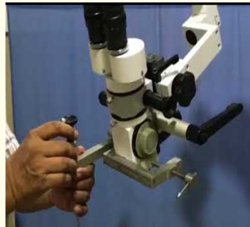
Figure 3: For 2 handed technique Justtache endoscope holder.
