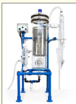
**Figure 1:** Laboratory-scale steam distillation apparatus.
