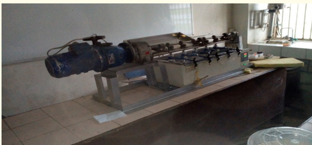
Figure 1: The fermentor used for liquefaction and saccharification.
