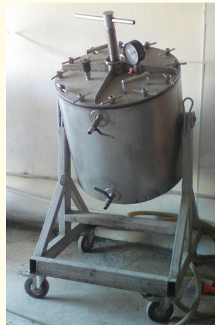
Figure 1: Universal module, working volume 75 dm 3 .
