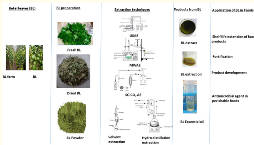
Figure 1: Betel leaves processing for extraction and its utilization in foods.
