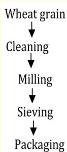
Figure 2: Flow sheet for the processing of wheat flour.
