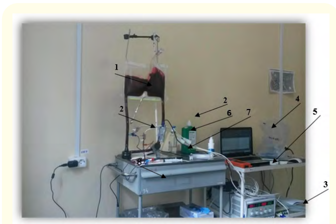
Figure 1: General view of the stand for studying the effect of a disk-type circulatory aid device on the parameters of donated blood. Symbols: 1 - blood tank; 2 - Tygon tubes; 3 - Biosoft-M device for pressure measurement; 4 - software on a laptop; 5 - flow meter; 6 - heat exchanger; 7 - screw clamp; 8 - disc pump.
