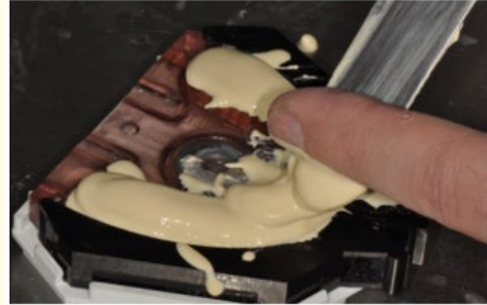
Figure 21: Working cast pouring.
