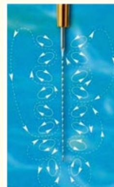
Figure 6: Acoustic streaming around a size 15 endosonic file. Depiction of the waves generated around the vibrating ultrasonic file (ACTEON North America/Clinical Research Dental) [35].
