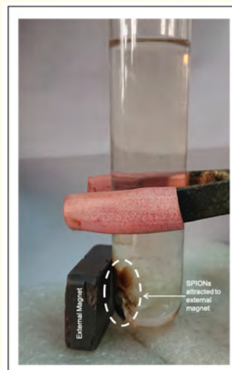
Figure 1: DC-SPIONs attracted to external magnet.
