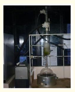
Figure 1: Soxhlet extraction unit.
