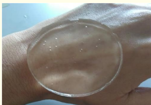
Figure 1: PVA / PVP hydrogel crosslinked by gamma radiation.
