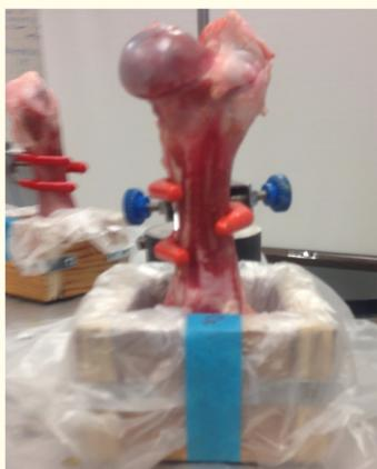
Figure 3: Fixated bone in wooden mold.
