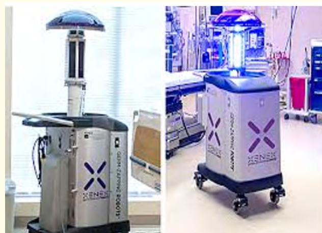
Figure 8: Xenex Germ-zapping Robot with LED Xenon bulb.
