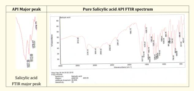
Figure 4: Pure Salicylic acid FTIR spectrum.
