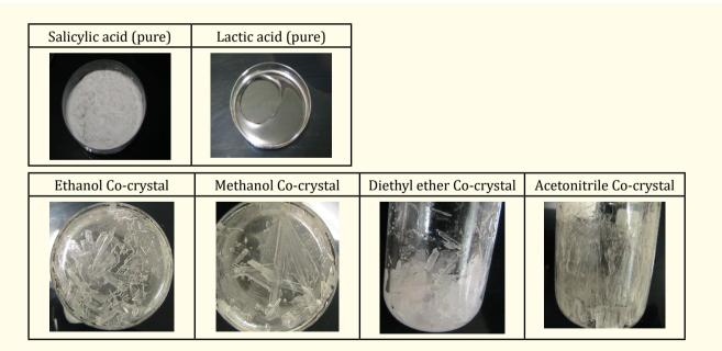
Figure 3: Co-crystals obtained from each co-solvent/Reflux technique.
