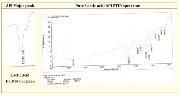
Figure 5: Pure Lactic acid FTIR spectrum.
