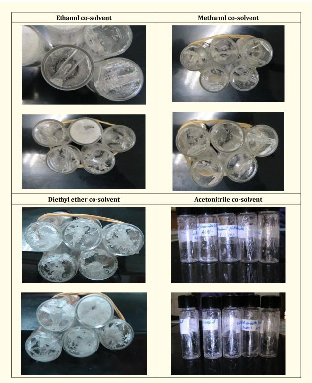
Figure 6: Co-crystal obtained from each co-solvent/grinding technique.
