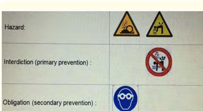
Figure 4: Workers’ perception [in the classroom]: the band saw risk is ejecting of materials, handling of materials.
