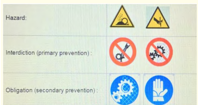
Figure 3: H&S manager’s perception: the band saw risk is ejection of materials, injuries, amputation.
