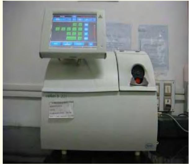
**Figure 3:** Shows Arterial blood gas analyser.
