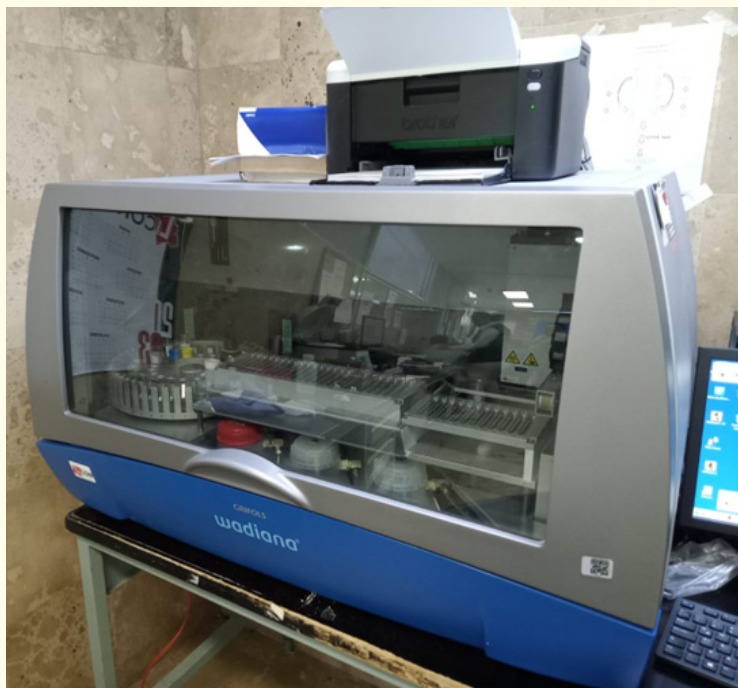
Figure 2: WADiana® equipment used to run blood types on gel cards.
