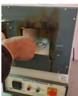
Figure: Determination of Ash Value using Muffle Furnace
