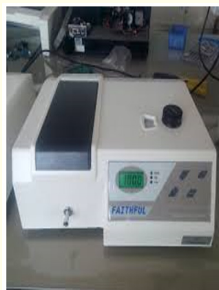
Spectrophotometer for detecting OD of serial dilutions.
