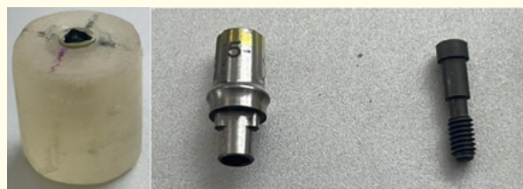
Figure 4: Trichannel implant embedded in acrylic material, conical and abutment screw.
