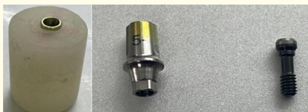
Figure 3: Conical implant embedded in acrylic material, conical and abutment screw.
