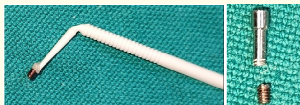
Figure 3: Retrieved Fractured Screw.
