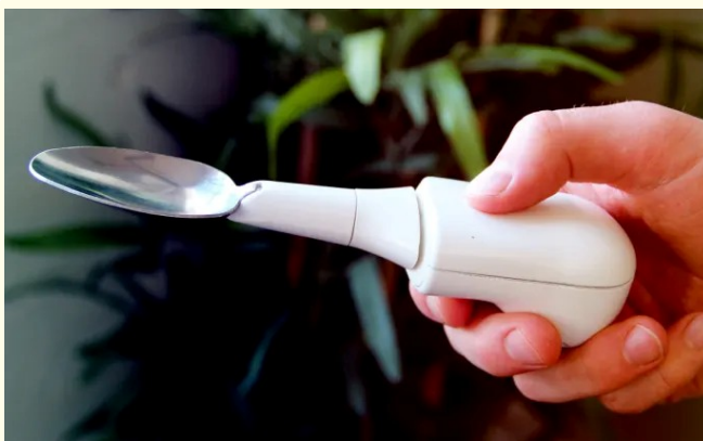
Figure 17: Stabilising electronic spoon for tremor patients.
