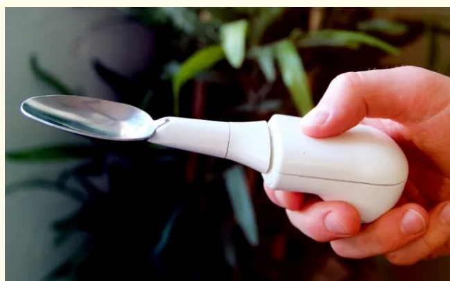
Figure 17: Stabilising electronic spoon for tremor patients.
