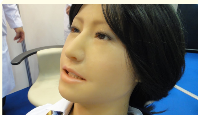
Figure 9: Dental training humanoid robot.
