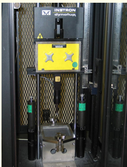
Figure 2: Drop weight impact tester.
