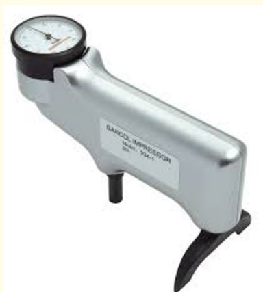
Figure 3: Barcol hardness tester.
