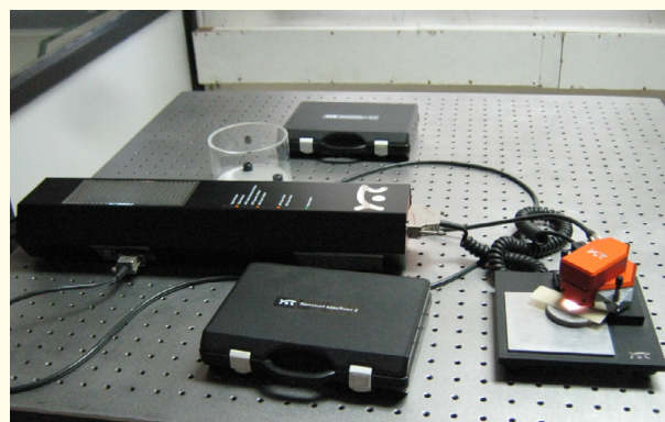
Figure 4: Atomic force microscopy assembly.
