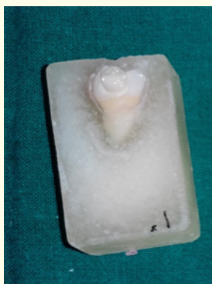
Figure 2: Prepared sample with GIC type II condensed in a cylindrical shape of 5mm diameter.
