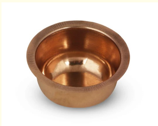
Figure 9: Copper vessel used to store distilled water and for immersing specimens to test the antimicrobial potential.
