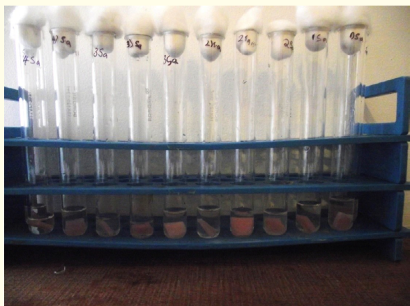
Figure 6: Inoculated specimens were placed in Phosphate Buffered Saline solution
