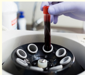
Figure 5: Balanced arrangement of tubes in the Kasvi centrifuge.
