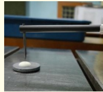
Figure 6: Contact angle measurement with chisel tip.
