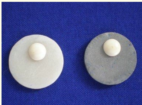
Figure 4a: Cement drops on the specimens.
