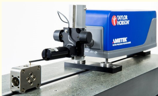
Figure 5: Contour and roughness tester for contact angle measurement.
