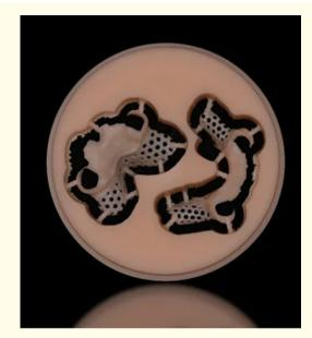
Figure 1: Milled polymer-based framework. (Source- Akl, M.A. and Stendahl, C.G.,2022).
