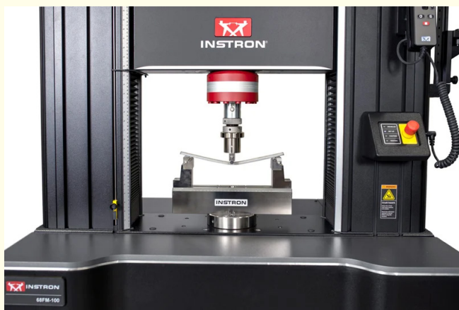
Figure 7: Three point bend test.
