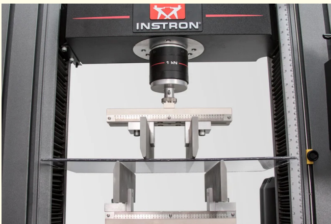
Figure 8: Four point bend test.
