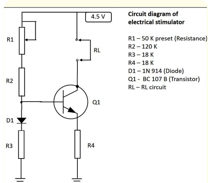
Figure 1: Circuit diagram of electrical stimulator.
