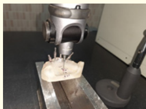
Figure 12: Coordinates measurement using CMM.
