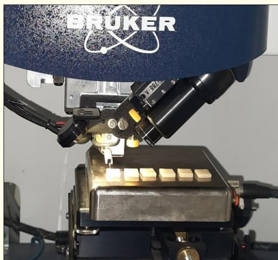
Figure 2: Measurement of surface roughness of uncoated Heat cure PMMA resin samples (Group IA) and CAD/CAM PMMA resin samples (Group IIA).
