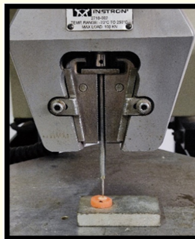
Figure 2: Push-out bond strength evaluation of slice mounted on lower segment of universal testing machine.
