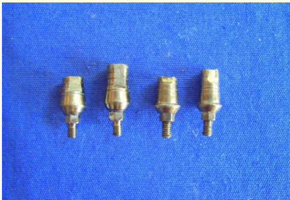
Figure 3: Abutments machined to 4mm and 6mm height.
