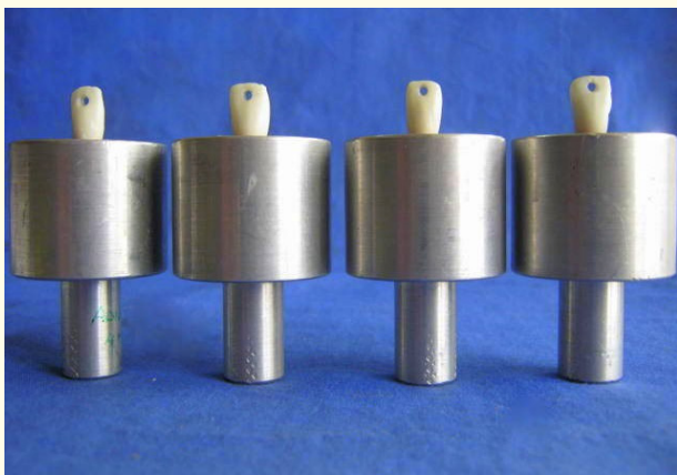
Figure 8: Zirconia copings cemented to the implant assembly.
