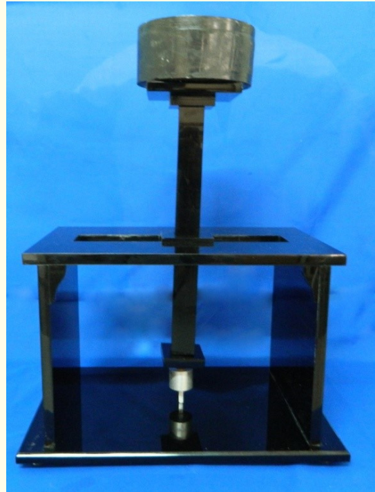
Figure 9: Cemented specimen loaded with a weight of 5kg.
