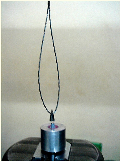
Figure 12: Dislodgement of the coping on application of tensile load.
