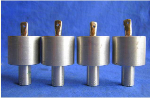
Figure 7: Metal copings cemented to the implant assembly.
