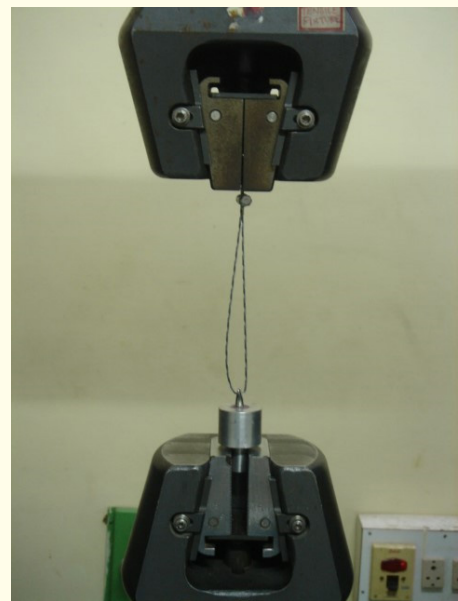
Figure 11: Specimen attached to the Universal testing machine with a wire loop.
