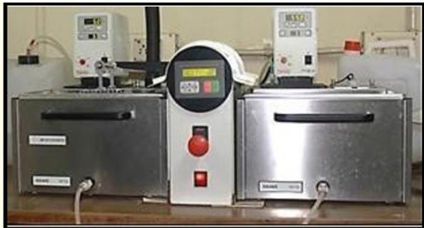
**Figure 9:** Thermocycling of Test Samples.
