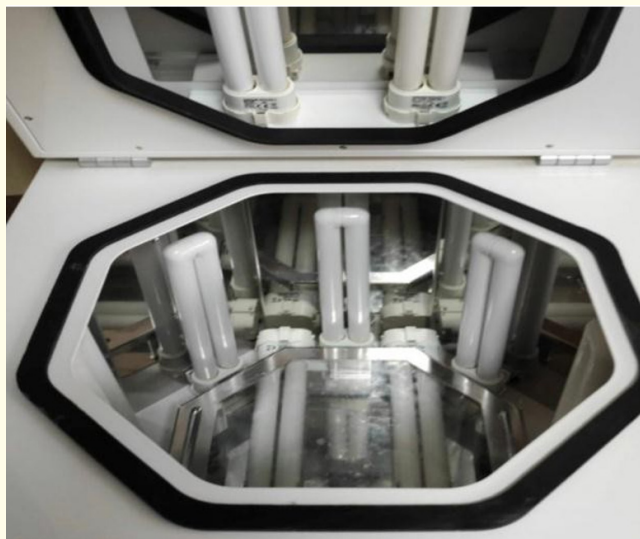
Figure 3: Group II samples in NEXTDENT 5100 post curing unit.
