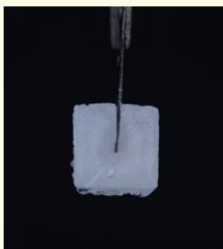
Figure 2: Slice passing through the center of the fiber post mold.
