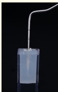
Figure 3: Packing of composite inside the transparent mold.
