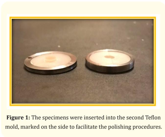
**Figure 1:** The specimens were inserted into the second Teflon mold, marked on the side to facilitate the polishing procedures.
