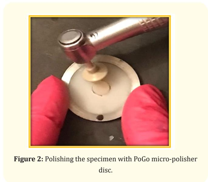
**Figure 2:** Polishing the specimen with PoGo micro-polisher disc.
