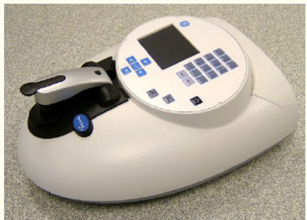
Figure 4: NanoDrop spectrophotometer to determine RNA concentration and purity.
