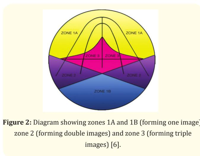
Figure 2: Diagram showing zones 1A and 1B (forming one image), zone 2 (forming double images) and zone 3 (forming triple images) [6].
